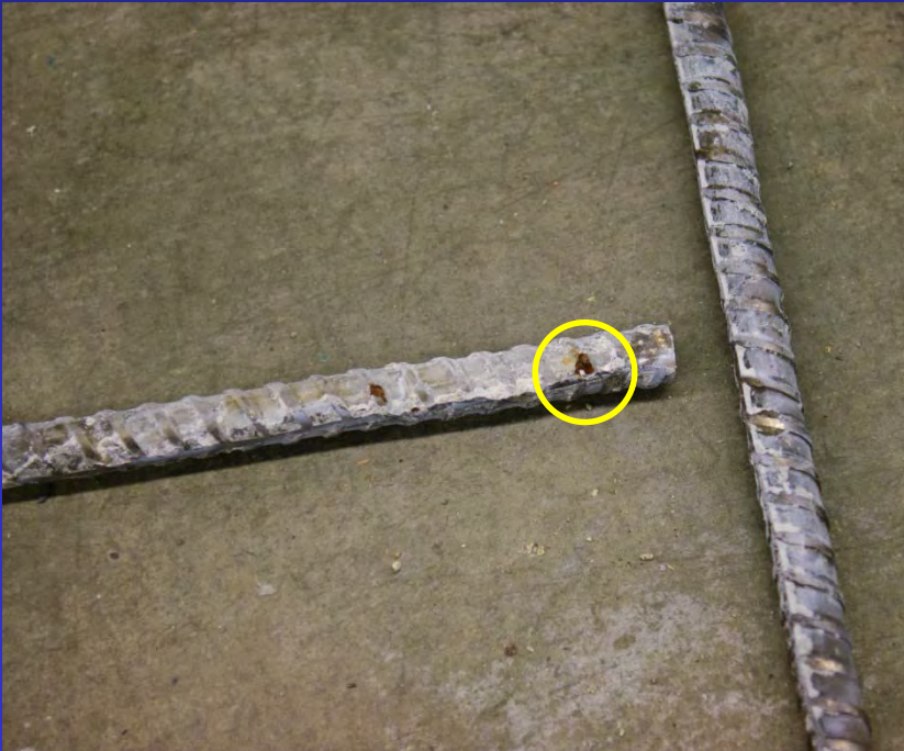
Discoloration and reddish-brown corrosion products
