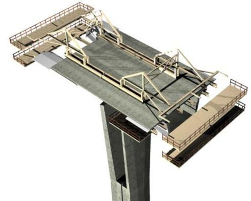
• The Form Travelers are constructed primarily of steel with some wood sections that can be cut to form the geometry of the segment
