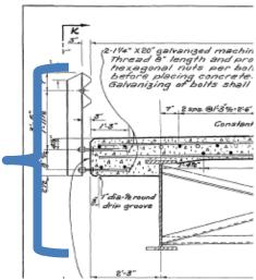
Figure 2 - Offset Distance in this example is not on the plans and needed field measured
